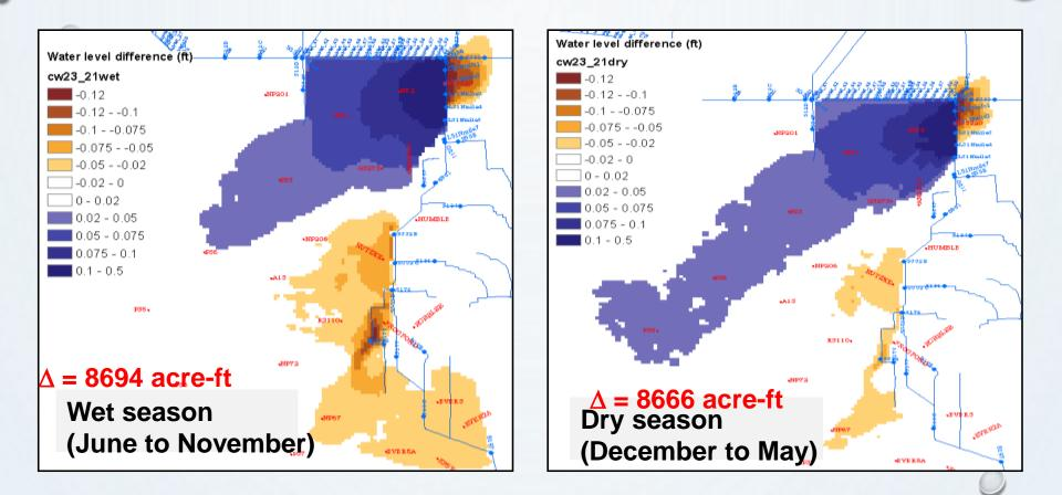
Curtain wall - 5-mile vs no wall Differences in surface water level
